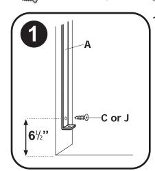
1. Install hinge bracket (A) to wall (stationary side of gate) using Phillips screw (C) beginning 6½" above floor surface. (Use ruler on left edge of this sheet to measure from floor).
