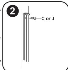
Install second screw (C) in top of hinge bracket securing it to the wall.
