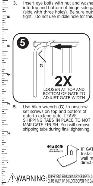
Use Allen wrench (G) to unscrew set screws on top and bottom of gate to extend gate. LEAVE SHIPPING TABS IN PLACE TO NOT MAR GATE FINISH. You will remove shipping tabs during final tightening.
