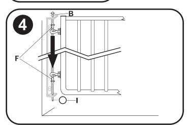
Hang gate by inserting hinge rod (B), through top of mounted hinge bracket (A), through upper plastic 4. shoulder washer (F), through both eye bolts, through lower plastic shoulder washer (F), and finally through bottom of hinge bracket. To secure hinge, insert key ring (I) through hole in end of hinge rod. Gate can be mounted at angles up to 30 degrees.
