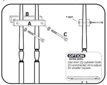
Insert bolt with washer through clamp and screw into T-nut on opposite clamp. The clamp with the T-nut should be on the outside of the post. Mount gate according to instructions. Use shim if necessary to account instructions. to ensure level gate installation.
