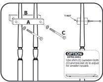
Insert bolt with washer through clamp and screw into T-nut on opposite clamp. The clamp with the T-nut should be on the outside of the post. Mount gate according to instructions. Use shim if necessary to accurate local each instruction. to ensure level gate installation.
