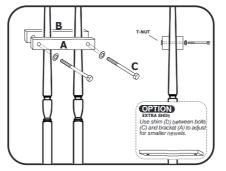
Insert bolt with washer through clamp and screw into T-nut on opposite clamp. The clamp with the T-nut should be on the outside of the post. Mount gate according to instructions. Use shim if necessary to ensure level gate installation.
